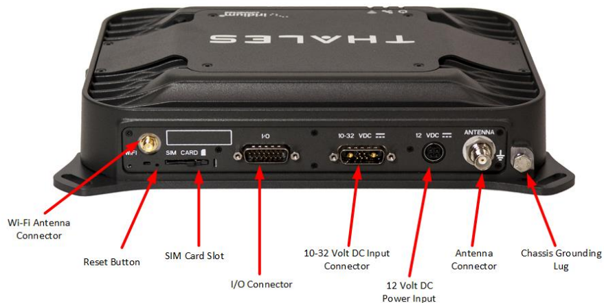
Figure 1-5 Below Deck Unit (BDU) Back Panel Detail
